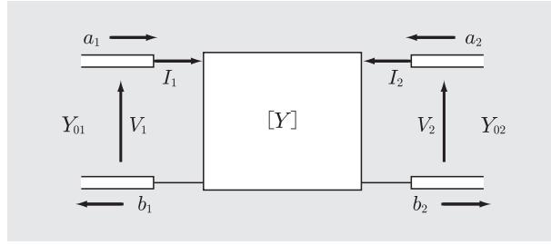
$$\begin{pmatrix} I_1 \\ I_2 \end{pmatrix} = \begin{pmatrix} Y_{11} & Y_{12} \\ Y_{21} & Y_{22} \end{pmatrix} \begin{pmatrix} V_1 \\ V_2 \end{pmatrix} \quad (1)$$
